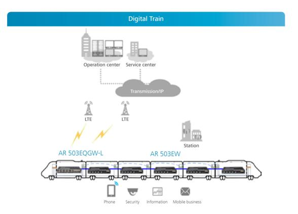
Deploy the AR503E on the train to provide a comprehensive solution for vehicle-ground communication, vehicle-mounted communication, and vehicle-mounted Wi-Fi coverage. Deploy the AR503EQGW-L on the front of the train to perform vehicleground communication through LTE links, and deploy the AR503EW on the train carriages to provide vehicle-mounted communication and Wi-Fi access.
